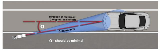
LPR accuracy is also dependent on the size of the characters on the image. For English characters, it is recommended to have an average of at least 16 pixel characters in height while for Arabic or other special characters; it is recommended to have 20 pixel height. In addition, large characters are not suitable for LPR. Try and avoid camera placements where the character size is greater than 50 pixels in height. Each character should be at least 2 pixels wide.
